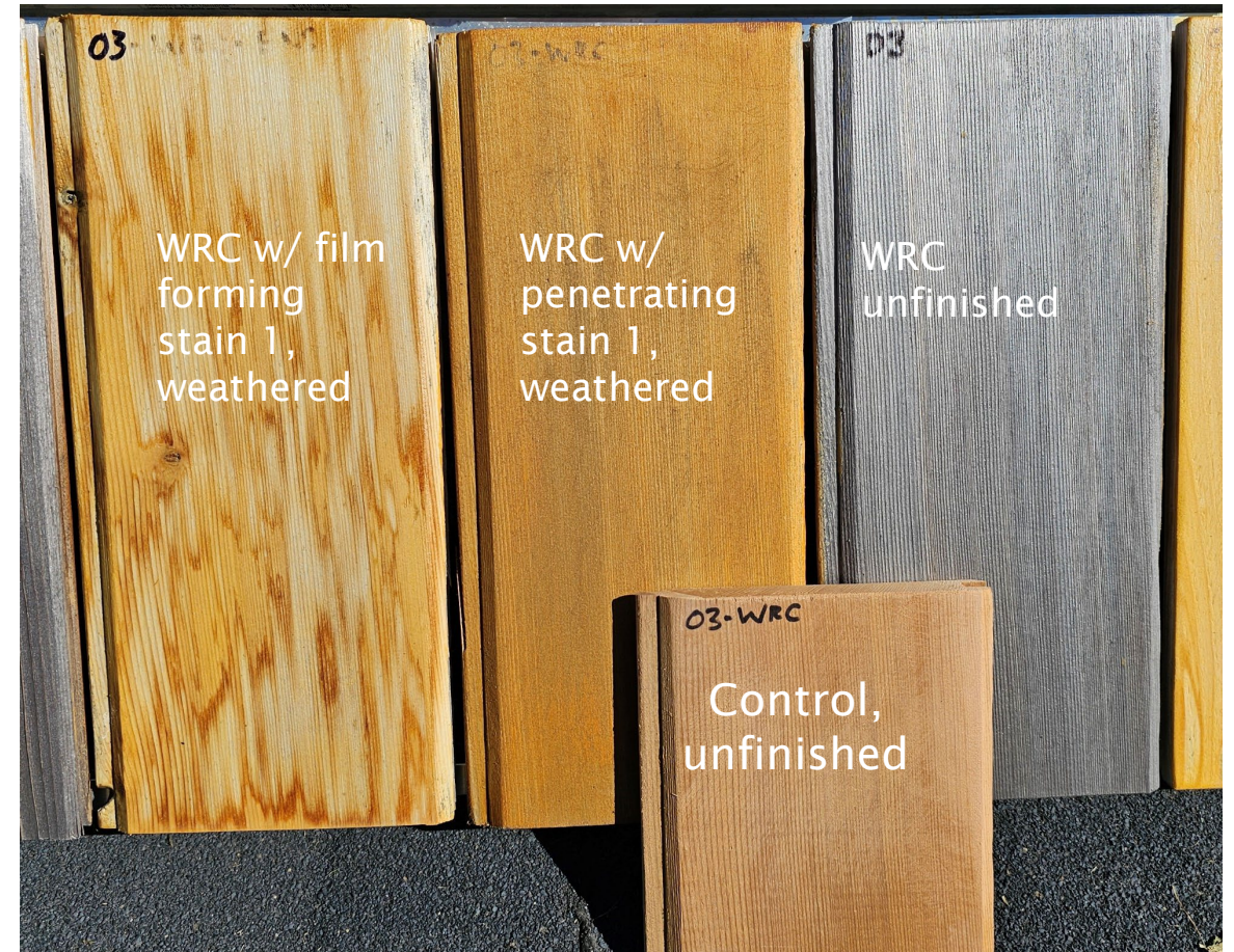
Example documentation at point in time (dated and is ongoing). Photo is showing the same three weathered samples vs control as in photo to the left from initial setup. Additional observations such as wood distortion, checking/splitting, fungal growth, finish deterioration etc are commented on as observed. Microscopic photos and spectrophotometer observations also taken at intervals
