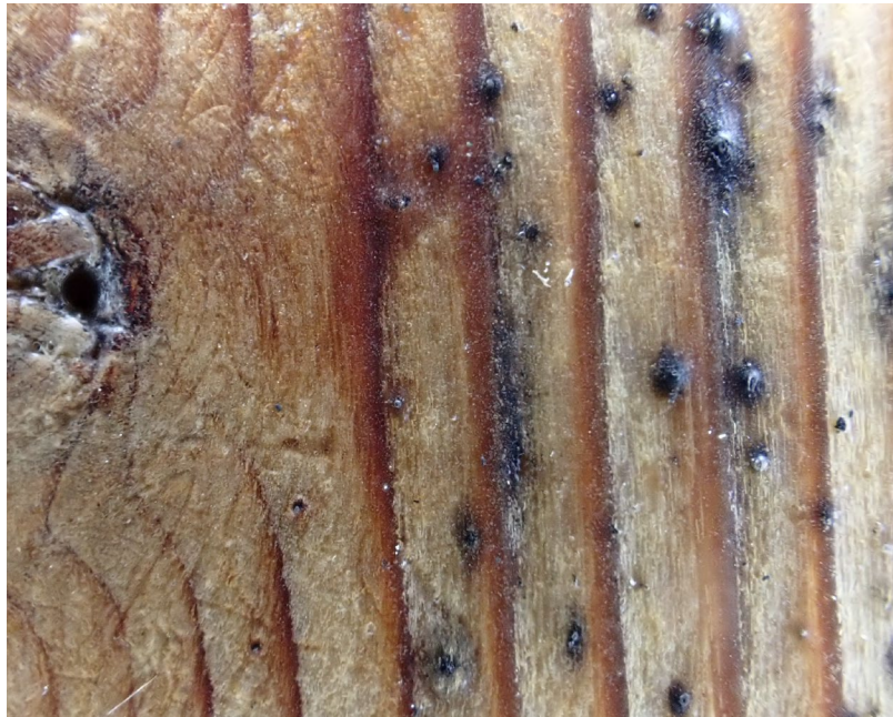
Film Forming Stain – Staining Fungi Underneath Stain in Wood Coating Still Hydrophobic
