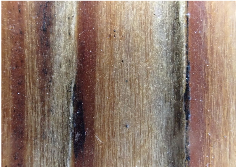
Film Forming Stain – Staining Fungi Underneath Stain in Wood Coating Still Hydrophobic
