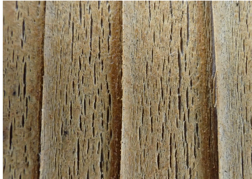
Penetrating Stain – Some surface fungi growth Note different stain penetration (with some residual on surface) between late and early wood grain Coating no longer hydrophobic Some raising of grain
