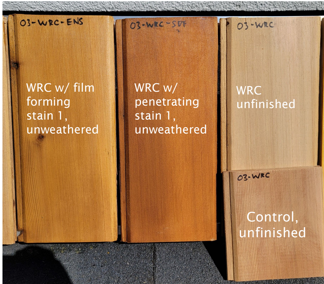
Initial Sample Setup, Un-weathered. Western Red Cedar (WRC) hence 03-WRC naming that is field finished with film forming stain 1 (left), penetrating stain 1 (middle), and unfinished (right). The control sample (lower right) is cut from same cladding pieces and its color and grain to represent the unfinished sample here
